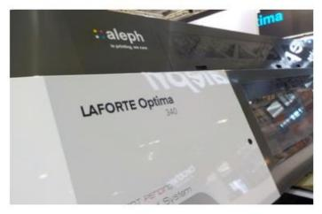
Aleph's new Optima 340 prints at up to 600sqm/hour in a single pass
